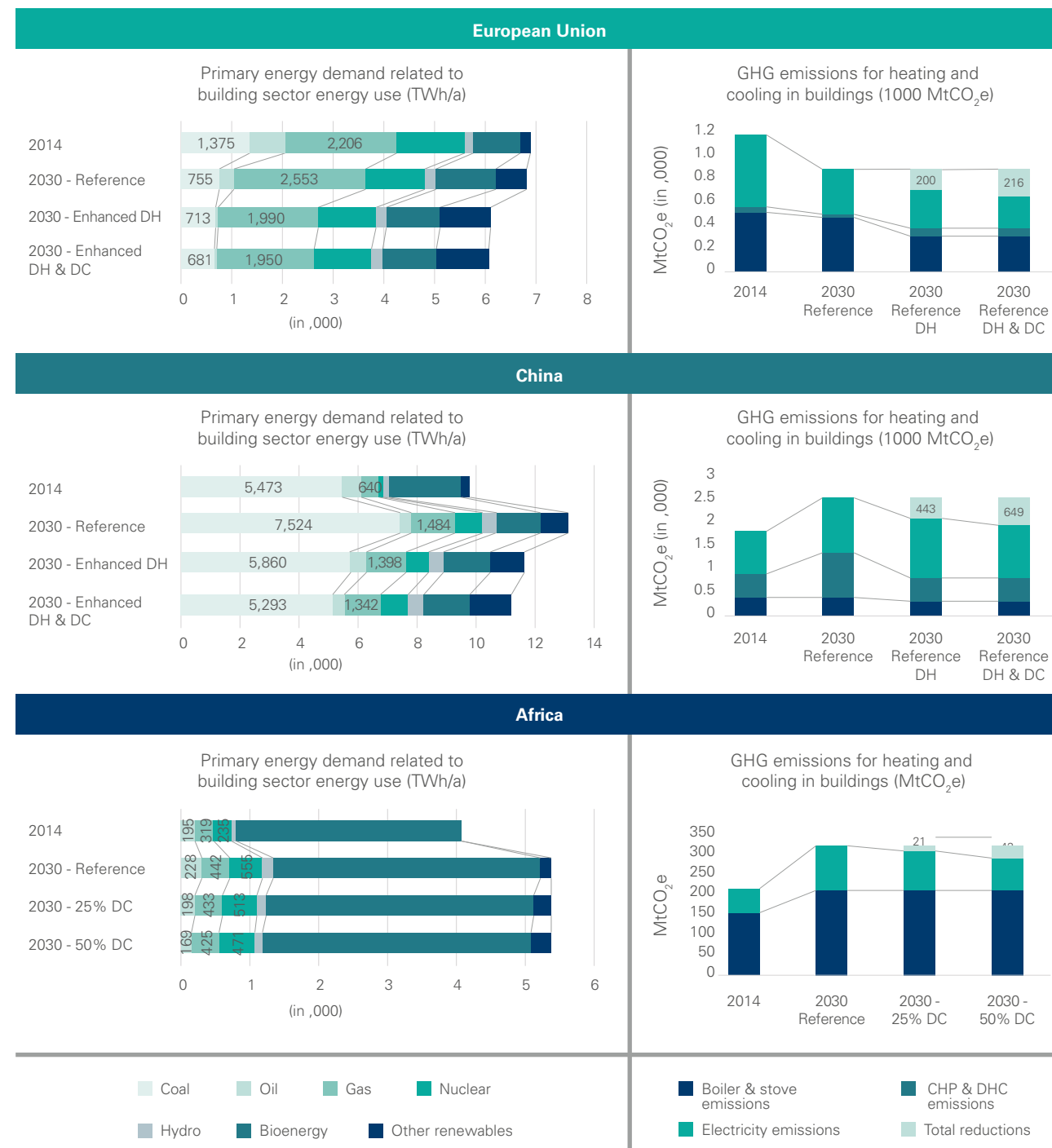
Figure 18: Primary energy demand for building sector energy use and GHG emissions for heating and cooling, under different scenarios.
